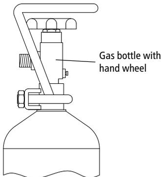
**Note:** The that the room where a carbon dioxide gas bottle is placed must have a minimum room volume of 38 m<sup>3</sup> for every kg of bottle capacity. At a one-kilogram bottle and an assumed room height of 2.2 m you will need at least 18 m<sup>2</sup> floor area.
