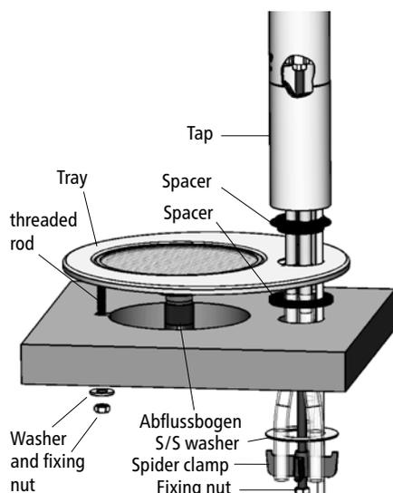
bend, turn it to the correct position and then tighten up the fastening nut again.
