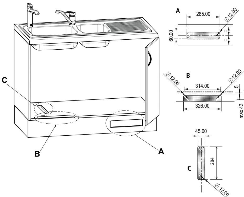
The cut outs A and B can be covered with the provided ventilation grilles.
