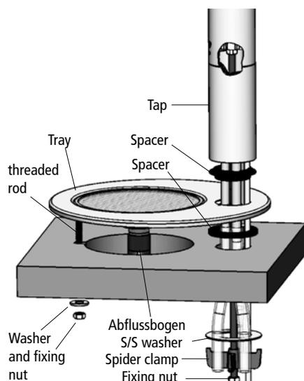
6. If the drain bend is facing the wrong way, slacken off the fastening nut above the bend, turn it to the correct position and then tighten up the fastening nut again.
