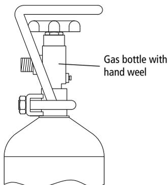
**Please note that the room where a carbon dioxide gas bottle is placed must have a minimum room volume of 38 m<sup>3</sup> for every kg of bottle capacity.**
