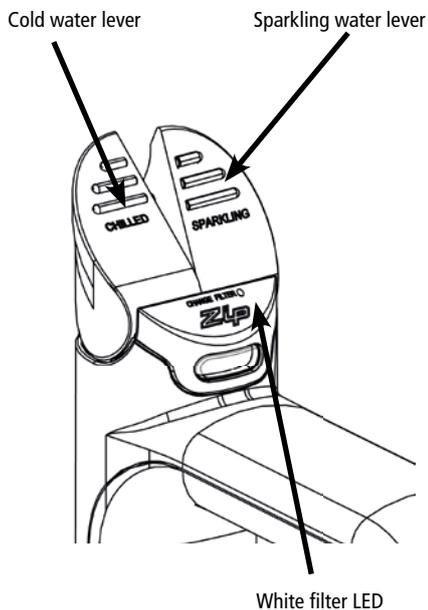
Press the blue "chilled" lever to dispense cold water. Pull the lever up to dispense cold water continually. The water will flow for 5 to 15 seconds. This time can be set in the menu. The lever then has to be manually returned to the Off position.
